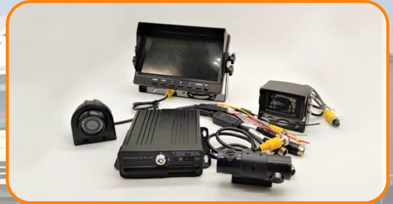
4 channel Mobile DVR system with 1080P high- resolution cameras + dual-lens DVR camera
