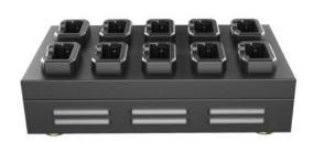
Police camera docking station is the latest charging and data uploading device, which can connect up to 10 cameras, via USB2.0 port. In addition to total power of docking reach 120 W, each port can provide up to 2.0A of self-adaption current, according to the connected devices. Users only need an office computer, without cumbersome wiring. It features multi-device data collection and charging. (Cameras not included)
